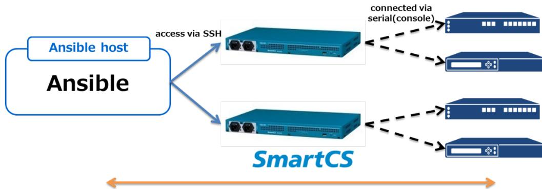
Previously, Telnet or SSH protocol had been used to connect to the SmartCS serial ports to directly execute operations manually. Using Ansible enables to execute operations automatically by creating a Playbook.
