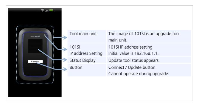
AP Firmware and more than one firmware such as Modem Firmware are in 101SI. Upgrade tool can upgrade AP Firmware and Modem Firmware.
